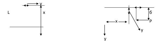
→ We Like to find out the minimum value of Load (P) for which the column isbuckled. → The minimum Load (P) is called critical Load/crippingLoad/Euler Load.
