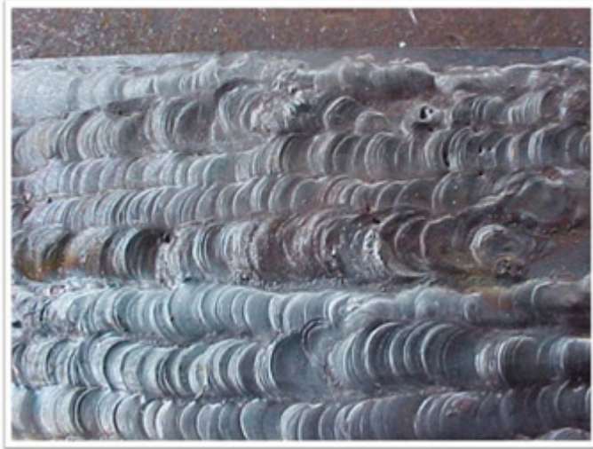
Figure 7.23 unacceptable weld profiles
