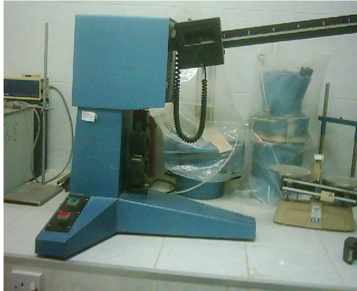
Fig. (3) The testing machine for cement mortar specimens in tension.
