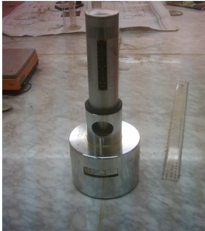
Fig.(21) The calibration of the Schmidt hammer.
