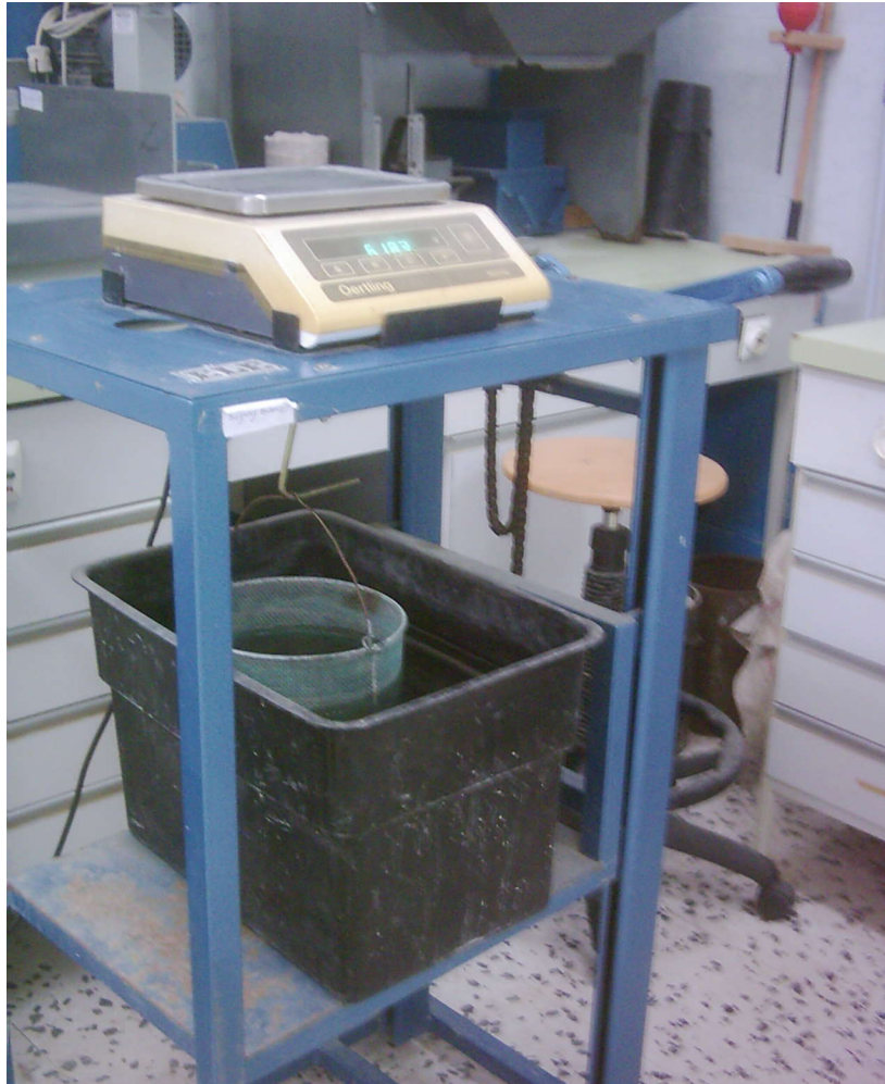
Fig.(3) A balance with suitable apparatus for suspending the sample container in water.
