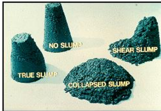
Fig. (9) Different possible slump test results.
