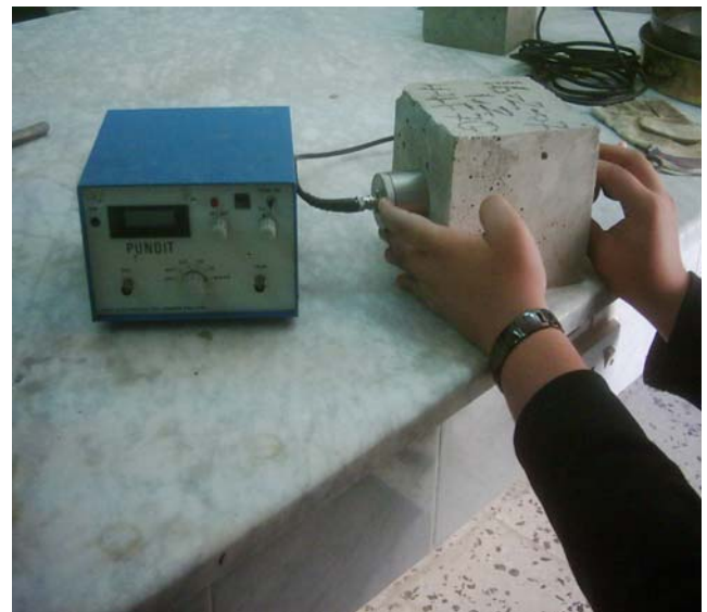
Fig.(24) Testing using PUNDIT
