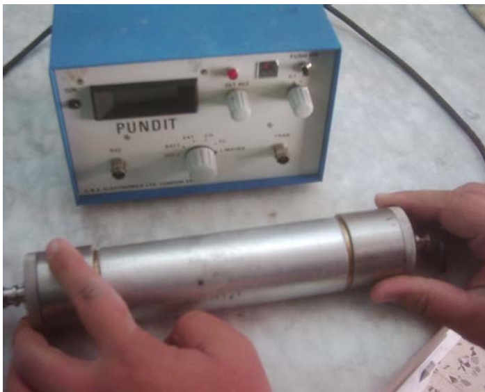
Fig.(23) The calibration of the PUNDIT.
