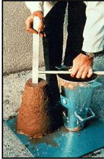
Fig.(8) Measuring the slump.
