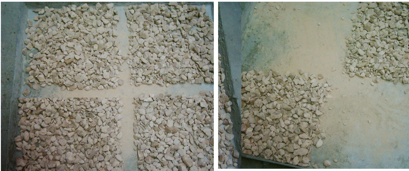
Fig.(2) Reducing Field Sample of Aggregate to Test Sample
