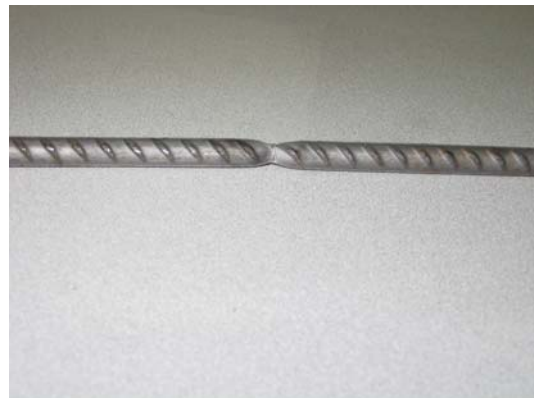
Necking of the rebar before fracture
