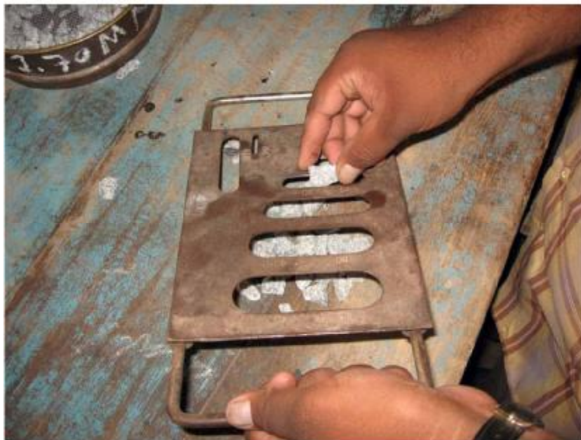
Flakiness Index Test in Progress
