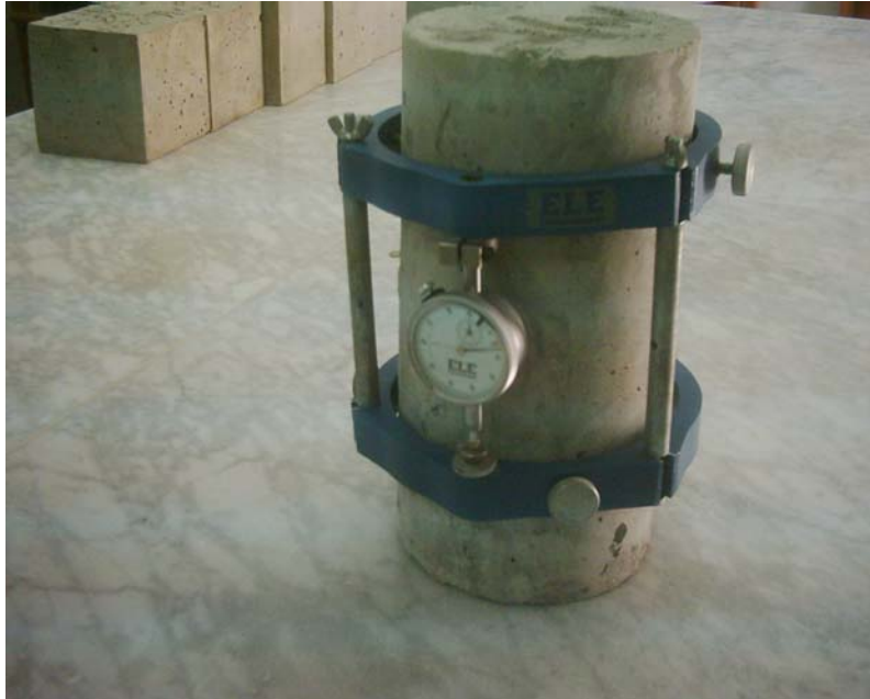
Fig. (26) Fixing the Compressometer for measuring the average deformation of the concrete cylinder.
