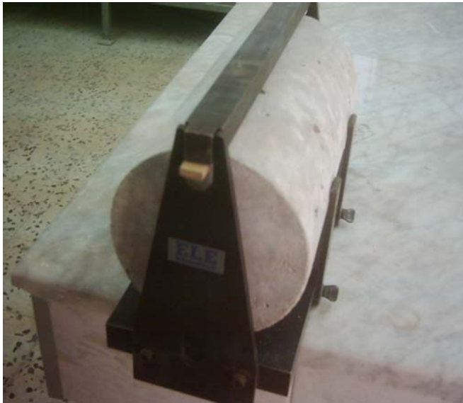
Fig.(19) The jig for aligning concrete cylinder and bearing strips
