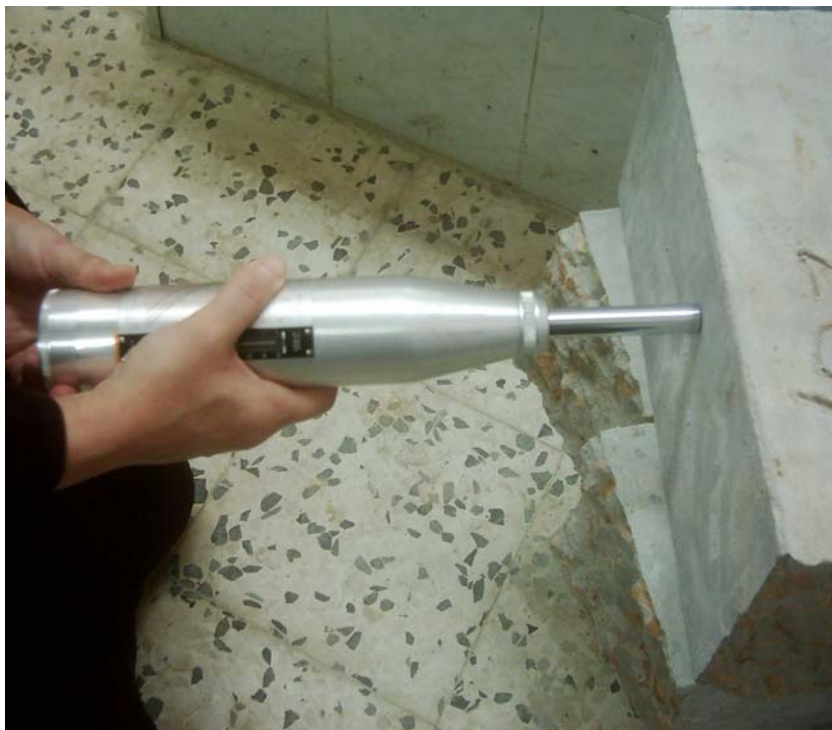
Fig.(22) Testing concrete using the Schmidt hammer.
