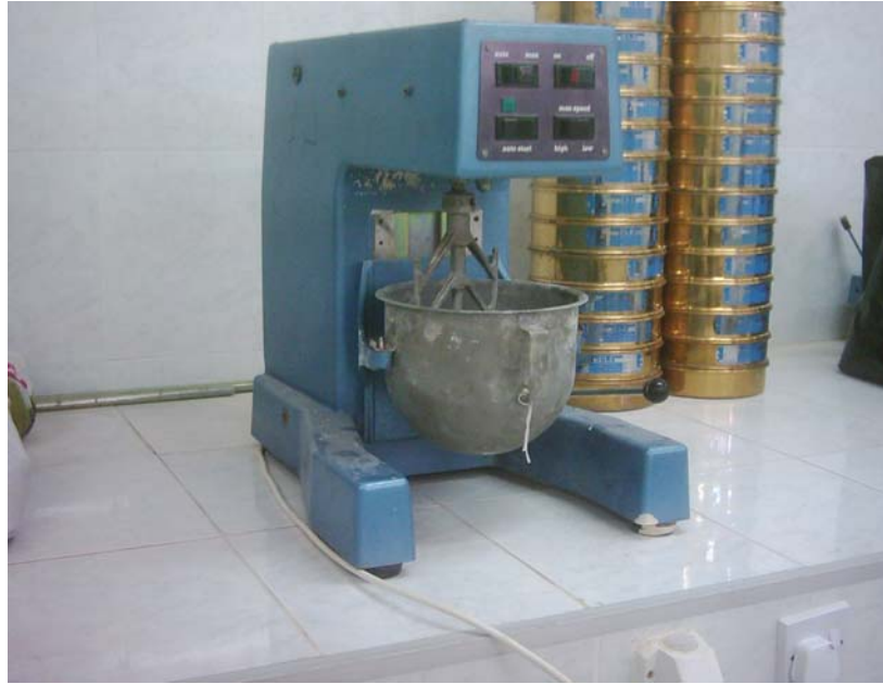
Fig.(1) The mixer to be used to mix the mortar.
