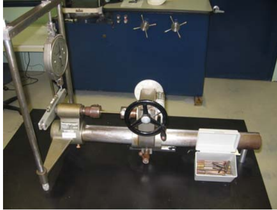
Figure 9: Torsion Testing Machine with bar specimens
