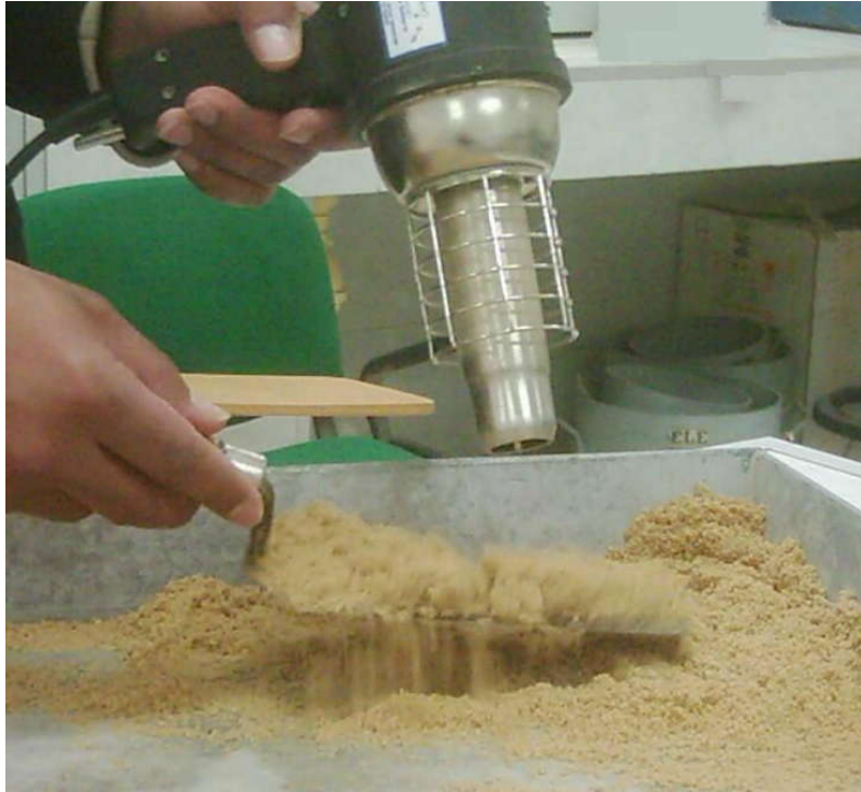
Fig.(4) Exposing the fine aggregate to a gently moving current of warm air.
