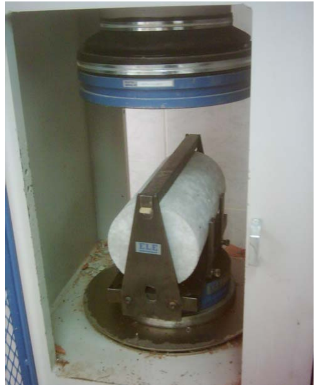
Fig.(20) Fitting the cylinder in the compression machine.
